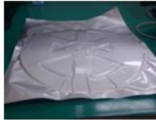
Squashed Reel as a Result of Vacuum Sealing
