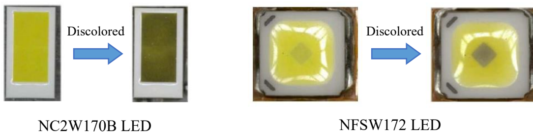
Figure 6. Examples of Discoloration due to VOCs
